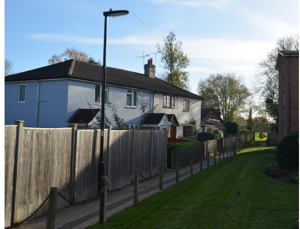
Figure 36: Local examples of street lighting with appropriate distance from the dwellings in order to avoid causing disturbance to the residents and light pollution.
