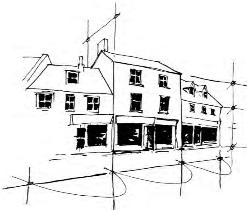
Fig 1.6 Sketch diagram illustrating the typical rhythms and relatively consistent key dimensions (see guidance table) along the town centre streets
